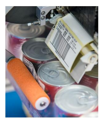
The correct method is often dictated by the surface texture and material of your outer packaging. For example, rougher surfaces typically need to use a tamp application method to ensure appropriate adhesion, as might a non-flat surface or 'lumpy' products (imagine a plastic bag of loose components).
