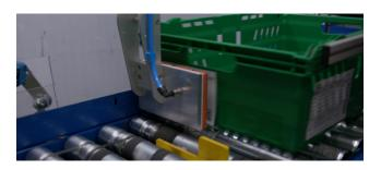
Secondary to the barcode labelling, each tote box is RFID tagged. This serves two purposes with the data on the tags linked to the barcode data to ensure that the correct items are sent to the correct customer, and so that the totes can be accounted for properly when they return.
